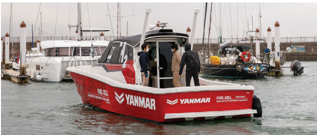
Yanmar engine test speed boat fuelled with hydrogen.
